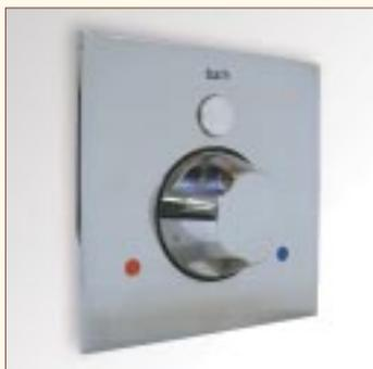
This unique wall mounted bathfiller has an anti-ligature easy-grip temperature control knob, linked directly to a recessed Thermostatic Mixer Valve (Type 3 DO8 NHS Approved). Bathfill is started by a Touch Sensor and stops automatically at the pre-selected level (a tamper-proof 'refill delay' setting is optional). Other features can include a divert to shower, and a 1/2 and full fill sensor option - all thermostatically controlled.
