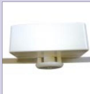
This version is for concealed ceiling mounting. The PIR detector is mounted in a thin disc of high density polyethylene and secured in the ceiling. The fixings and controls fit into the ceiling void out of sight.
