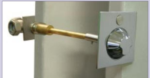
A combination of thermostatic shower temperature control and Touch Sensor, with an anti-ligature temperature control knob. The high quality mixer\* is securely held in the duct space and supported on brackets. \*Meeting Type 2 or DOH/ Type 3 specifications.
