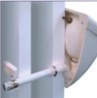
This easy to install sensor system is concealed behind the bowl and when used, initiates the flush cycle for that bowl alone, independent of other bowls in the range. This is a highly water efficient, hygienic and totally vandal resistant flushing system, with long term maintenance benefits.
