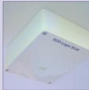
This PIR controller fits neatly on the ceiling or side walls, and senses the approach area in front of the urinals. The frequency of flush cycles is fully adjustable to meet Bye-law demands, and push button commissioning and set up makes for very simple installation. Battery life typically 4-5 years.
